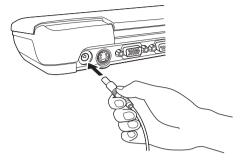
Figure 3-3 Connecting the adaptor to the computer
